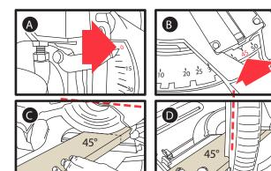
We recommend using a compound miter saw fitted with a carbide tipped cross blade (60 or 80 teeth, ATB) for cutting the Stair Nose molding.
